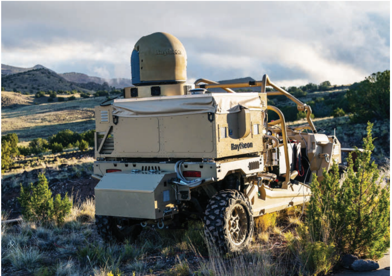
Raytheon's Multispectral Targeting System (MTS) combines optical and infrared sensors to acquire and track airborne targets and direct the laser beam it fires. For C-UAV, the MTS was modified to track Class-1 drones (under 20 pounds) and Class 2 drones (between 20 and 55 pounds), the most common sizes used by terrorists and insurgents.
