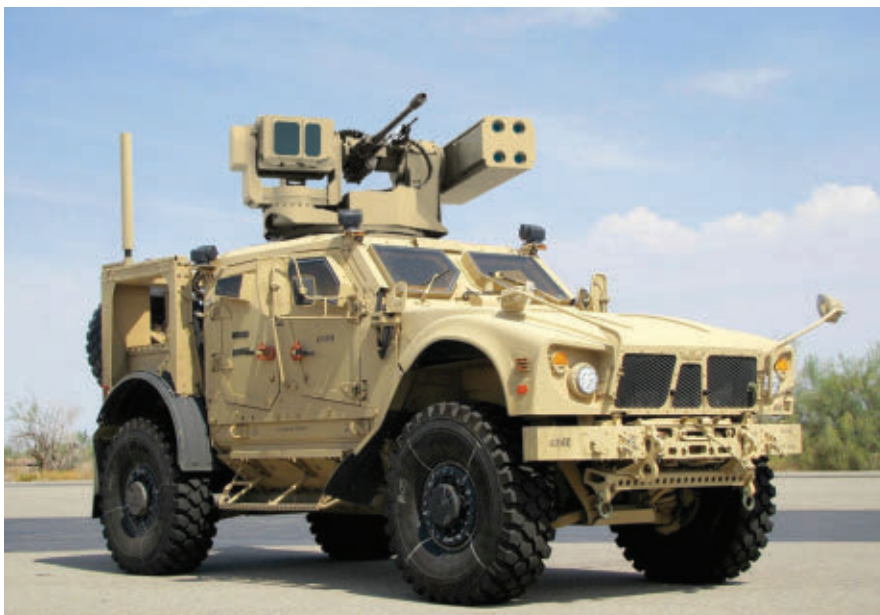
Leonardo DRS is developing the vehicle-mounted Mobile Low, Slow Unmanned Aerial Vehicle Integrated Defense Systems (MLIDS) to disable small drones.
