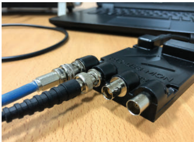
The Abaco palm-sized BT3-USB-MON MIL-STD-1553 avionics databus monitor is for flight line databus test applications.
