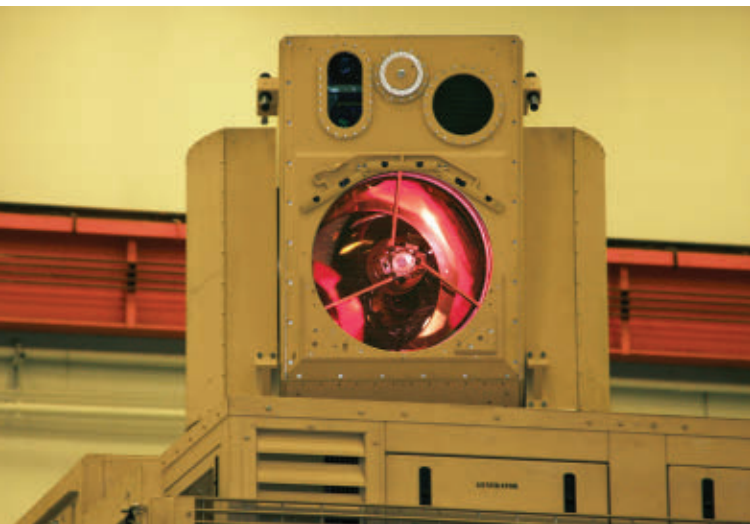
The Boeing High Energy Laser Mobile Demonstrator (HEL MD), developed originally to protect forward-deployed warfighters from rockets, mortars, and artillery shells, is yielding laser weapons technology to counter unmanned aerial vehicles.
